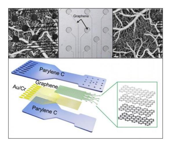
Conventional metal electrode technologies (top left) are opaque, obstructing views of underlying neural tissue. DARPA's RE-NET program has developed new graphene sensors that are electrically conductive but only 4 atoms thick—hundreds of times thinner than current contacts (top middle). Their extreme thinness enables nearly all light to pass through across a wide range of wavelengths. Placed on a flexible plastic backing that conforms to the shape of
