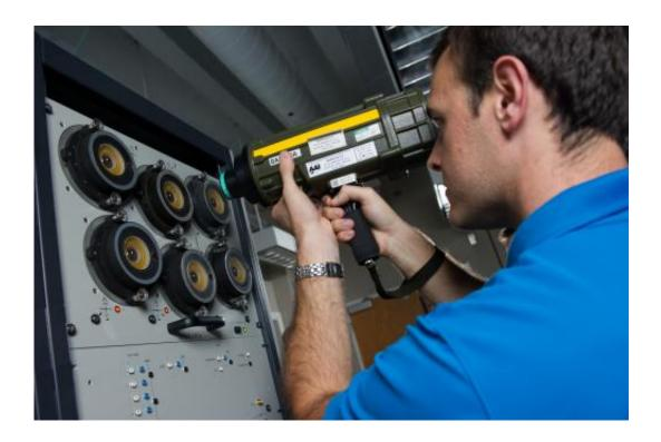
GTRI researcher Michael Coulter stimulates the AN/AAR-57 Common Missile Warning System integrated support station to evaluate the system's response to a simulated threat. GTRI and the Army Reprogramming Analysis Team (ARAT) developed and built a new integrated support station (ISS) to test software updates. Credit: Rob Felt
