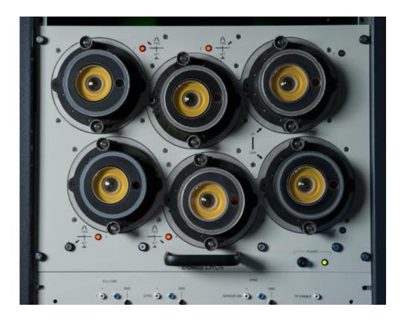
Sensors used in the AN/AAR-57 Common Missile Warning System are part of the integrated support station developed to test system software updates. GTRI and the Army Reprogramming Analysis Team (ARAT) developed and built a new integrated support station (ISS) to test software updates. Credit: Rob Felt)
