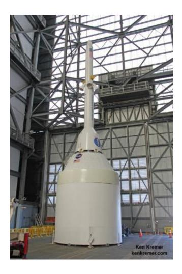
Orion crew capsule, Service Module and 6 ton Launch Abort System (LAS) mock up stack inside the transfer aisle of the Vehicle Assembly Building (VAB) at the Kennedy Space Center (KSC) in Florida. Service module at bottom. Credit: Ken Kremer/kenkremer.com
