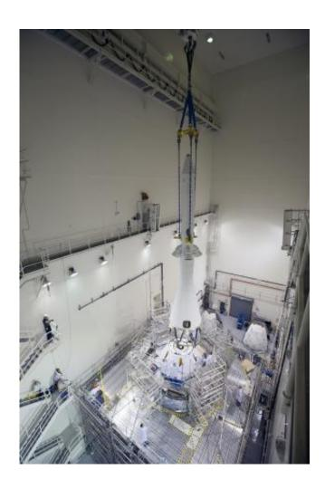
The launch abort system is lowered by crane for installation on the Orion spacecraft for Exploration Flight Test-1 inside the Launch Abort System Facility, or LASF, at NASA's Kennedy Space Center in Florida. Credit: NASA/Cory Huston
