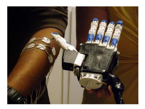
The 3D-printed prosthetic hand can be programmed to recognize a hand at-rest, open-faced, closed (tool grip), a three-finger grip, and fine pinch. Credit: Mike Koon, University of Illinois
