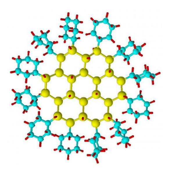
At left, a structural model of a typical silicon nanocrystal (yellow) stabilized within an organic shell of cyclohexane (blue). At right, a high-resolution transmission electron microscope photograph of a single silicon nanoparticle. Credit: NIST
