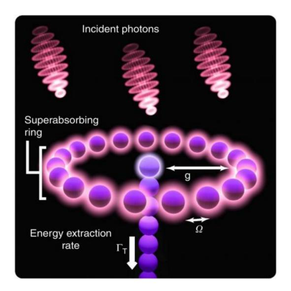
In one potential method to realize superabsorption, a superabsorbing ring absorbs incident photons, giving rise to excitons. Credit: Higgins, et al.
