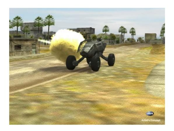
One of the key goals of DARPA's Ground X-Vehicle Technology (GXV-T) program is improving the survivability of ground-based armored fighting vehicles by increasing vehicle agility. Vehicle agility involves
