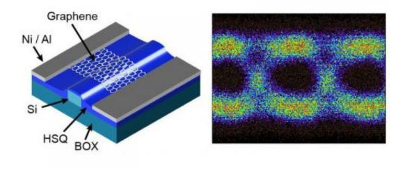
In cooperation with Alcatel Lucent Bell Labs researcher from AMO realized the worldwide fastest Graphene based photodetectors. By demonstrating a maximum data rate of 50 GBit/s a new record level could be reached, pushing this technology closer to applications.
