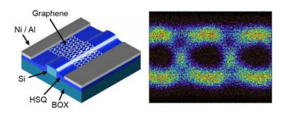
In cooperation with Alcatel Lucent Bell Labs researcher from AMO realized the worldwide fastest Graphene based photodetectors. By demonstrating a maximum data rate of 50 GBit/s a new record level could be reached, pushing this technology closer to applications.
