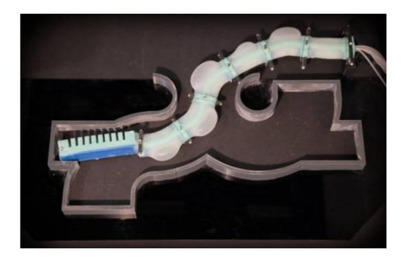
The CSAIL team's rubber robotic arm moves using pressurized air that causes it to change shape like a balloon. Credit: Jason Dorfman, CSAIL
