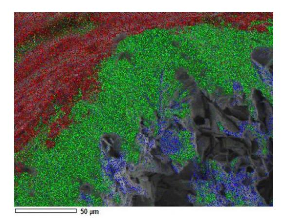
Energy dispersive x-ray spectroscopy image was taken within a scanning electron microscope, illustrating a Bi2212 wire shown in blue and green, coated with the titania-based insulation shown in red. Credit: Sasha Ishmael
