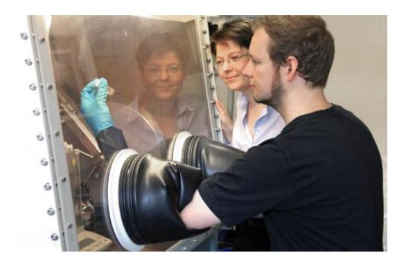
Most syntheses were carried out under exclusion of air and moisture. For this purpose, the Institute of Organic Chemistry has a glove-box, which contains nitrogen as a chemically inert protective atmosphere. In front: Julian Linshöft, at the back: Anne Staubitz. Credit: Grace Suana
