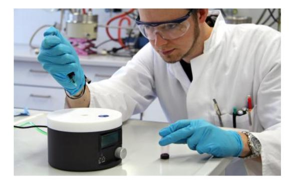
The polymer can be processed from solution to form a thin film. The technology, which is used here, is called spin coating. A solution is being dripped onto a fast rotating disc and the solvent is flung away. In the photo: Julian Linshöft is preparing a polymer film. Credit: Grace Suana
