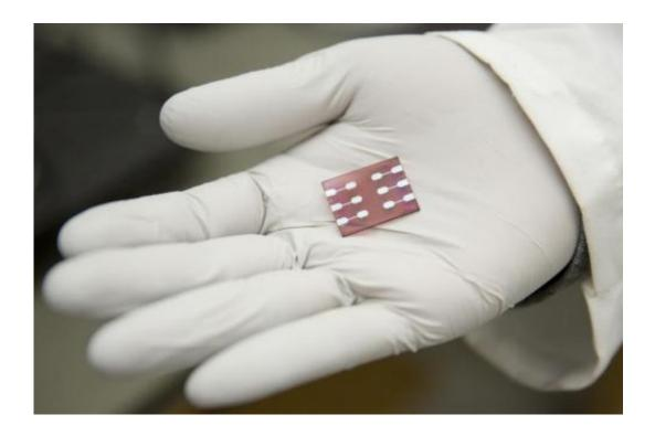
This polymer solar cell consists of a new polymer, called PID2, which was developed in the laboratory of Luping Yu, professor in chemistry at the University of Chicago. The new polymer improves the efficiency of electrical power generation by 15 percent when added to a standard polymer-fullerene mixture. Credit: Andrew Nelles
