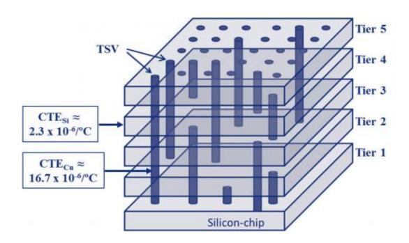
Schematic diagram of a three-dimensional stacked integrated circuit (3D-SIC), achieved using copper through-silicon via (TSV) interconnects. The large mismatch in the coefficient of thermal expansion (CTE) between copper TSV and surrounding Si leads to large stress build-up.
