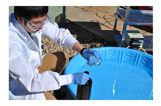
In this image, University of Alberta civil engineering graduate student Zengquan Shu simulates the solar UV/chlorine treatment process. Laboratory-scale tests found the solar UV/chlorine treatment process removed 75 to 84 per cent of the toxins found in oil sands process affected water. Credit: UAlberta Civil and Environmental Engineering
