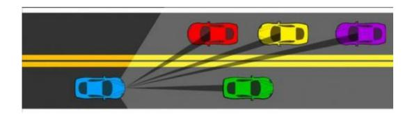
A smart headlight system developed at Carnegie Mellon University is able to track other vehicles on the road and selectively block light that would otherwise reach the eyes of other drivers. Credit: Carnegie Mellon University Robotics Institute
