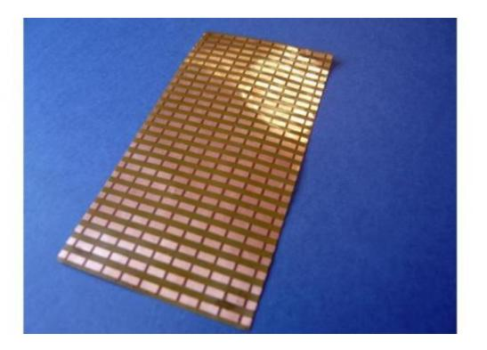
The fabricated AMC. The longest dimension of each unit cell is 40% smaller than equivalent designs
