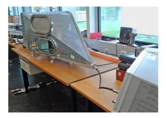
In the lab: the set-up used for the reflection coefficient measurements of the AMC
