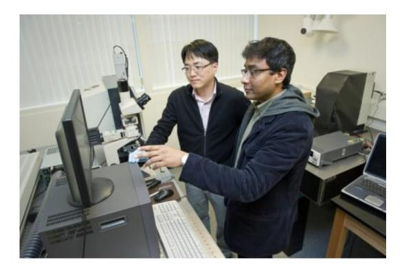
Swastik Kar (right), and Yung Joon Jung use a Raman Spectrometer to characterize the assembly of a carbon nanotube. Credit: Mary Knox Merrill
