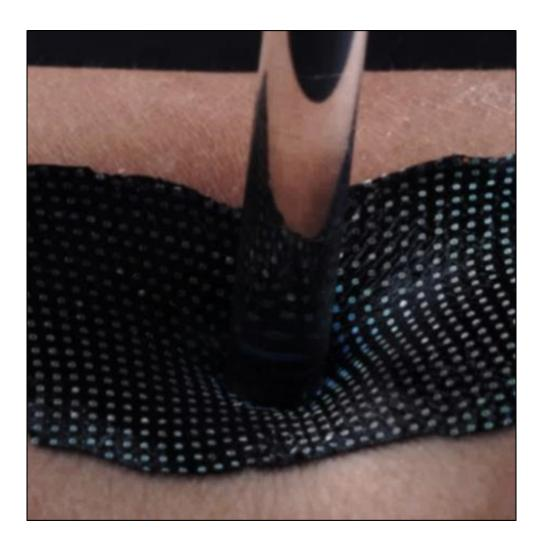
A new photonic device for health monitoring is as flexible as the skin on which it is placed. The comfortable device can alert the wearer to any heart trouble or dry skin. Credit: John A. Rogers, University of Illinois
