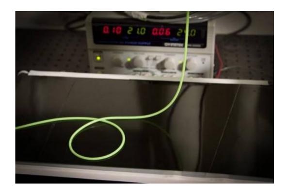
Desktop-scale experiment used to explore the various possible patterns obtained when a thin polymer rod (in green) is deployed onto a moving substrate (black conveyer belt). In this example, the rod forms a periodic array of loops in alternative directions. Credit: John Freidah/MIT
