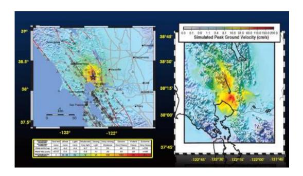
Researchers are using data from the South Napa earthquake to help validate models. These figures compare the (left) observed intensity of ground motion from seismic stations of the California Integrated Seismic Network "ShakeMap" with the (right) simulated shaking (peak ground velocity) from SW4 simulations using UC Berkeley Professor Doug Dreger's source model and the USGS 3D geologic/seismic model. Both figures use a similar color scale, though they cover different spatial domains.
