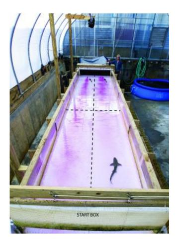
A smooth dogfish swims in a flume at Woods Hole Oceanographic Institute in Massachusetts. Arrows point to the brick baffles and the source of the food odor plume. The start box holding area is also labeled. Dashed lines indicate the flume quadrants used to determine activity level through number of lines crossed. Credit: Danielle Dixson
