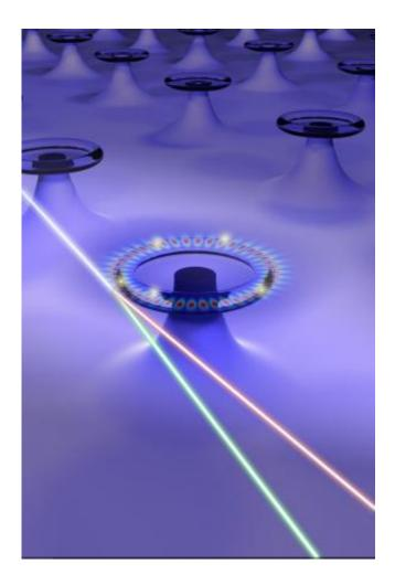
Arrays of self-referenced and self-heterodyned Whispering-Gallery Raman microlasers for single nanoparticle detection. A "pump" laser generates a single Raman lasing mode inside the silica resonators. Upon landing of a nanoparticle on the resonator, Raman laser circulating inside the resonator undergo mode splitting leading to two new lasing modes in different colors. Monitoring the changes in the color difference (frequency difference) enables detecting and
