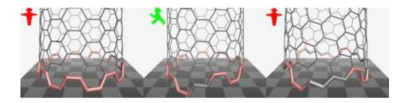
This graphic shows the difference between an armchair nanotube, left, with a fast-growing near-armchair nanotube, center, which has a single kink at its base. At right, a nanotube with multiple kinks is not as likely to grow under given conditions, according to a new formula for nanotube growth. Credit: Evgeni Penev
