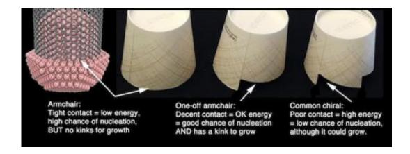
Coffee cups represent three types of carbon nanotubes analyzed by theoretical physicists at Rice University. The researchers determined that near-armchair nanotubes in a batch grow in the greatest bulk because they strike the most favorable balance between energy and speed. Nanotubes with a greater chiral angle, like the one at right, are not as favored because the high energy of the loose contact lowers the nucleation rate. Credit: The Yakobson Group
