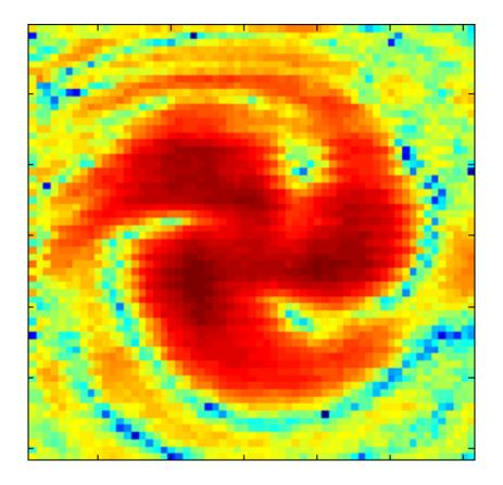
A graphic showing the intensity of the radio beams after twisting Credit: Alan Willner / USC Viterbi
