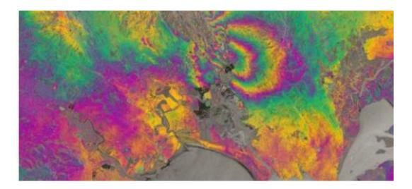
A radar interferogram from Sentinel-1A showing how the ground moved in the Napa Valley earthquake. Each coloured fringe is caused by a change in distance between the ground and the satellite of about 3cm. The extent of the ground deformation in the interferogram shows that the fault slip which occurred in this earthquake continues further north than the extent of the mapped rupture at the surface. Credit: Copernicus data (2014)/ESA/PPO.labs-Norut–COMET-SEOM Insarap study
