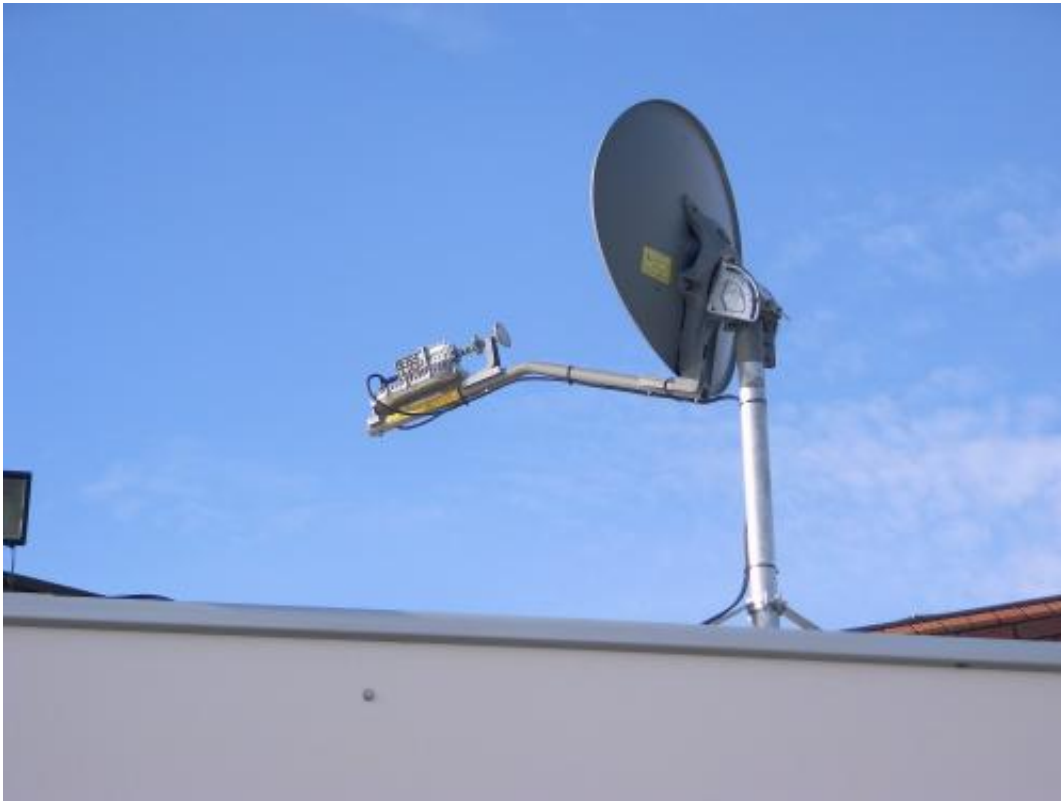
Self-pointing satellite dish on van. Credit: ESA
