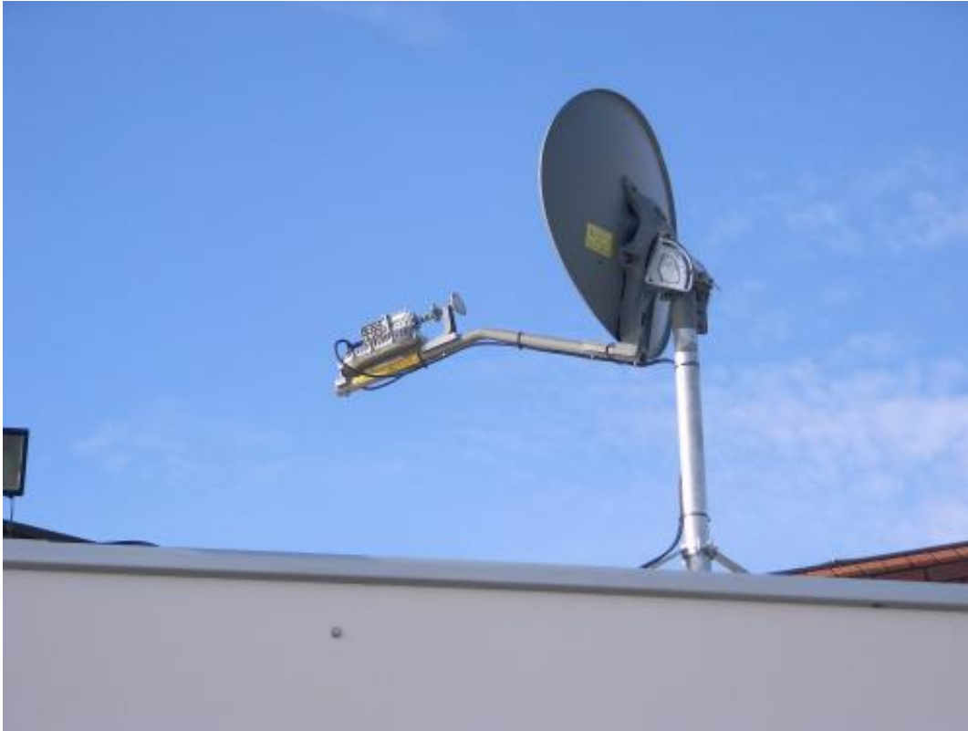
Self-pointing satellite dish on van. Credit: ESA
