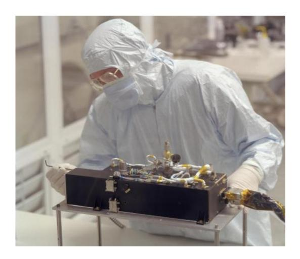
The Alice ultraviolet imaging spectrometer will be the first to study a comet up close. The shoebox-sized instrument is one-third to one-half the mass of comparable UV instruments, yet with more than 10,000 times as many imaging pixels as the spectrometer aboard Galileo. Credit: Southwest Research Institute
