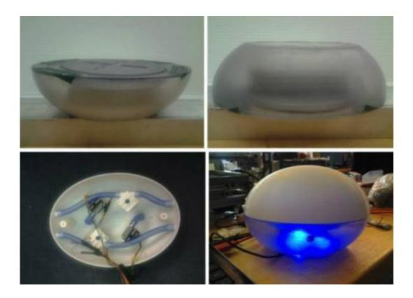
In the robot's watertight chamber are its control circuitry, its battery, a communications antenna, and an inertial measurement unit, which consists of three accelerometers and three gyroscopes that can gauge the robot's motion in any direction.
