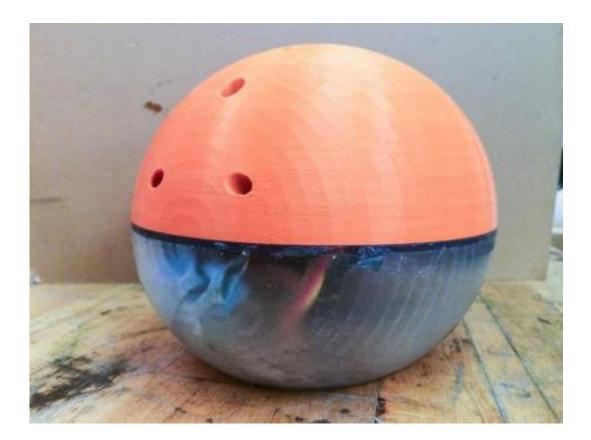
Half of the robot is waterproof and houses the electronics. The other half is permeable and houses the propulsion system, which consists of six pumps that expel water through rubber tubes. The main structural components of the robot were made with a 3-D printer.
