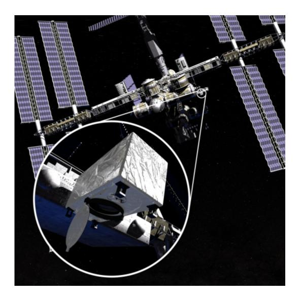
This artist's rendition of the Cloud-Aerosol-Transport System (CATS) shows its location on the International Space Station, where it will measure the character and worldwide distribution of the tiny particles that make up haze, dust, air pollutants and smoke in the atmosphere. Credit: NASA
