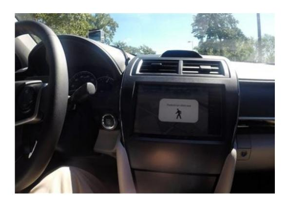
In a Monday, Sept. 8, 2014 image from video, an indicator on a digital display in a car detects a pedestrian walking nearby during a demonstration hosted by Denso at the Intelligent Transportation Society's World Congress in Detroit. The auto parts supplier is working on technology that uses smartphones to signal drivers if someone is walking into their path. (AP Photo/Mike Householder)
