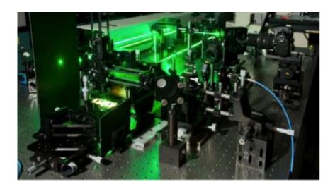
Experimental set-up researchers used to analyze the behavior of quantum dots placed on metal oxides. A laser illuminated the quantum dots to make them glow and a spectrometer was used to analyze the light they emitted. Credit: Seyed Sadeghi/ University of Alabama, Huntsville
