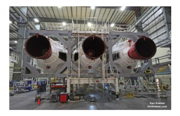
These three RS-68 engines will power each of the attached Delta IV Heavy Common Booster Cores (CBCs) that will launch NASA's maiden Orion on the EFT-1 mission in December 2014. Credit: Ken Kremer
