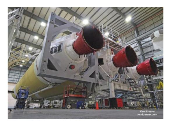
Side view shows trio of Common Booster Cores (CBCs) with RS-68 engines powering the Delta IV Heavy rocket resting horizontally in ULA's HIF processing facility at Cape Canaveral that will launch NASA's maiden Orion on the EFT-1 mission in December 2014 from Launch Complex 37. Credit: Ken Kremer
