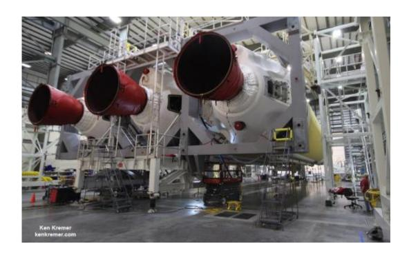
A United Launch Alliance technician monitors the core booster elements of a Delta IV Heavy rocket after being integrated in preparation for Exploration Flight Test-1 at Space Launch Complex 37 on Cape Canaveral Air Force Station. Credit: Ken Kremer
