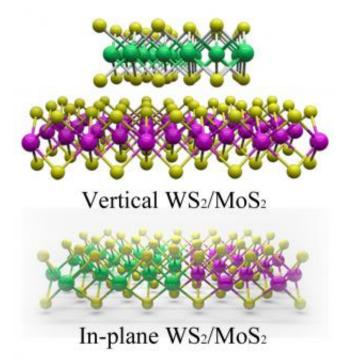
Stacked (top) and in-plane nanomaterials self-assemble in two ways, depending on the temperature at which they're grown, according to Rice University researchers who led the project. The semiconducting materials show promise for a new generation of "pixel" electronics. In the illustration, green spheres are tungsten, purple are molybdenum and yellow are sulfur. Credit: Ajayan Group/Rice University
