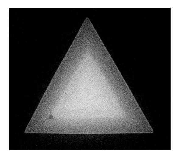
An image of an in-plane heterostructure of tungsten disulfide and molybdenum disulfide, created in an experiment at Rice University. The structures self assemble in a furnace at 650 degrees Celsius. Higher temperatures formed stacked heterostructures. The structure is about 20 microns across. Credit: Ajayan Group/Rice University
