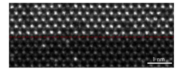
This atomic-resolution image shows the sharp line between tungsten disulfide (brighter) and molybdenum disulfide (darker) in a new material made in a collaboration led by Rice University. The two-dimensional material shows promise for nanoelectronic applications. Credit: Oak Ridge National Laboratory
