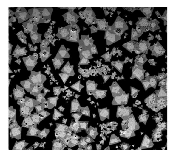
Stacked heterostructures of tungsten disulfide and molybdenum disulfide were grown in experiments at Rice University. The form of the structures depends on the growth temperature: Higher temperatures resulted in stacked structures, while lower temperatures produced in-plane structures. The material may be useful for nanoelectronic applications. Credit: Ajayan Group/Rice University
