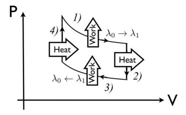
Scientists have devised a way to run a quantum cycle based on the use of quantum shortcuts to adiabaticity, where friction-like effects are quenched. Shown are the four steps of a quantum Otto cycle, where heat enters (exits) the working medium and those where work is performed by (done onto). Credit: A. del Campo, et al. ©2014 Nature *Scientific Reports*
