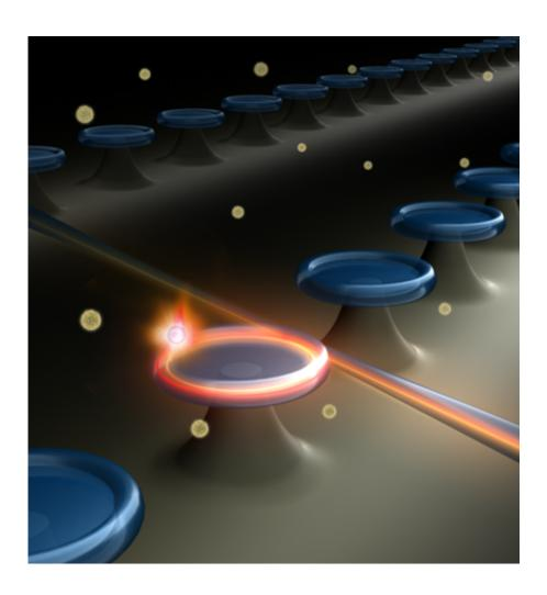
An array of microcavity Raman lasers for single nanoparticle detection. The pump laser light (in orange) is coupled into the microcavity via a fiber taper to generate the Raman laser (in red). When the Raman laser encounters a nanoparticle, it splits into two lasing lines due to backscattering, thus producing a beat note in the temporal Raman power. By measuring the beat frequency changes, real-time single nanoparticle detection can be performed.
