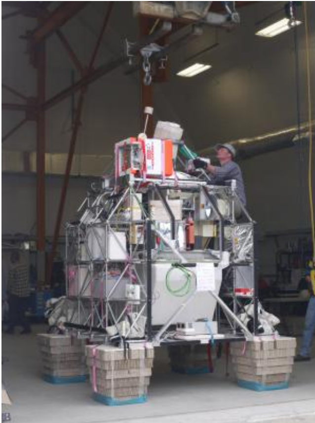
MIPAS gondola with remote sensing instruments. Credit: Hermann Oelhaf, KIT
