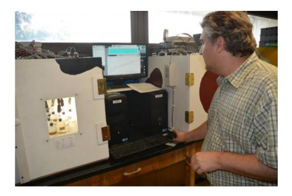
At Texas A&M, in support of the LRNS and CVDS models, Dr. Luis Tedeschi has developed in vitro gas production systems to assess digestion characteristics and biological values of feeds based on their pattern of accumulated gas during incubation with rumen fluid under anaerobic conditions. Credit: Blair Fannin
