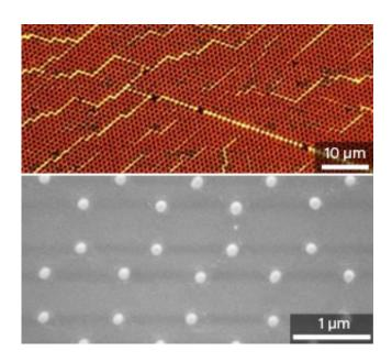
Dark-field microscopy (top) and scanning electron microscopy (bottom) images showing an array of plasmonic nanoparticles used as a highly sensitive sensor. Credit: Kalashnikov et al.
