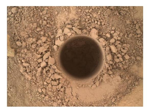
This image from the Mars Hand Lens Imager (MAHLI) camera on NASA's Curiosity Mars rover shows the first sample-collection hole drilled in Mount Sharp, the layered mountain that is the science destination of the rover's extended mission. Credit: NASA/JPL-Caltech/MSSS
