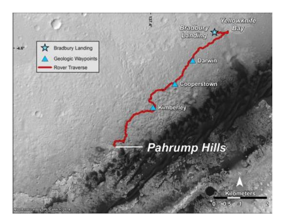
This map shows the route driven by NASA's Curiosity Mars rover from the "Bradbury Landing" location where it landed in August 2012 to the "Pahrump Hills" outcrop where it drilled into the lowest part of Mount Sharp. The rover reached Pahrump Hills with a 73-foot (22.4-meter) drive on the 653rd Martian day, or sol, of the rover's work on Mars (Sept. 19, 2014). Credit: NASA/JPL-Caltech/Univ. of Arizona
