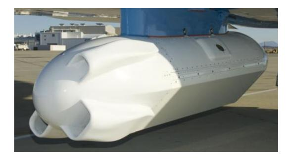
A close-up view of the pod housing JPL's sophisticated synthetic aperture radar system carried by NASA's C-20A Earth science research aircraft. Credit: NASA Armstrong
