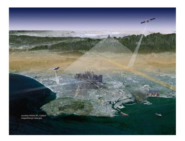
Artist's concept of the LA Megacities Carbon Project observing system. Ground sensors atop towers and buildings measure carbon dioxide, methane and carbon monoxide. An instrument atop Mt. Wilson scans the basin multiple times daily. Aircraft, mobile laboratories and satellites round out the network. Credit: NASA/JPL-Caltech
