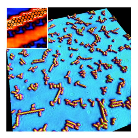
Graphene nanoribbons are fabricated by molecular assembly on a Cu(111) substrate. On this surface system, GNRs on grow in six azimuthal directions exclusively. White lines in the inset highlight the zigzag edges of a ribbon. Credit: Patrick Han
