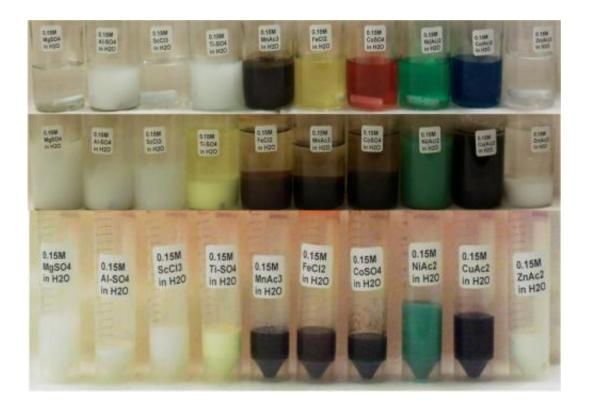
This figure illustrates the ease with which grams of many different types of oxide nanoparticles can be prepared in a single step. The first row of sample vials shows the initial salt solutions of the different elements. The second row shows the product after reaction with potassium superoxide (KO2) and the addition of methanol. The bottom row shows the grams of nanoparticles after being purified by centrifugation. Credit: U.S. Naval Research Laboratory
