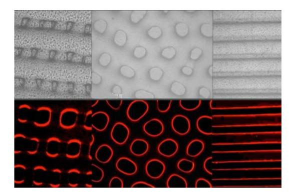
Images show textures (top) and fluorescent light (bottom) produced by the new synthetic elastomer material that can mimic some of the camouflage abilities of octopuses and other cephalopods.
