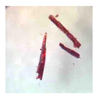
The crystalline material changes color when absorbing or releasing oxygen. Crystals are black when they are saturated with oxygen and pink when the oxygen has been released again. Credit: University of Southern Denmark
