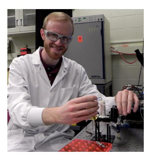
MIT graduate student Michael G. Christiansen with a magnetometry coil used to confirm heat output from magnetic iron oxide nanoparticles. Credit: Denis Paiste/Materials Processing Center
