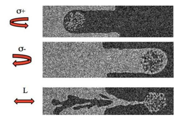
Images of magnetic domains in a cobalt platinum (Co/Pt) alloy multilayer film exposed to laser light where dark gray indicates one magnetization orientation, while the light gray indicates an opposite orientation. The images show that the final direction of magnetization can be controlled using circularly polarized light without the use of magnetic fields.
