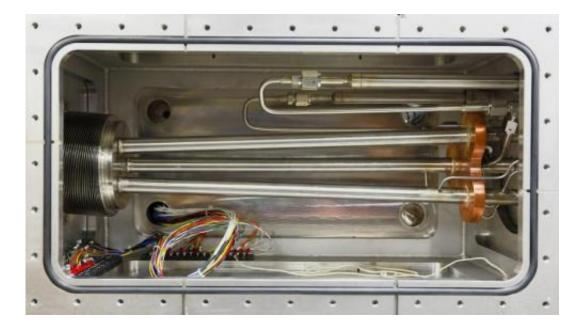
A three-barrel pellet injector developed at Oak Ridge National Laboratory for the ITER disruption mitigation system. Credit: US ITER/ORNL
