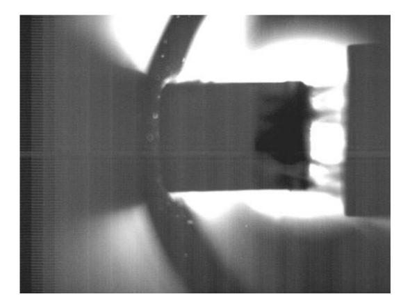
A 16 mm neon-deuterium pellet, indicated by an arrow, captured with a high speed camera as it travels from left to right at about 300 meters per second in a test stand at the Oak Ridge National Laboratory Pellet Lab. Credit: ORNL
