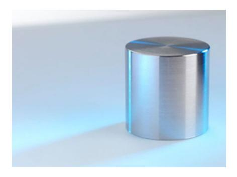
The UK national standard kilogram removed from its protective casing
