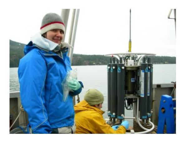
Researchers aboard the MSV John Strickland use a CTD rosette – an instrument suite measuring salinity, temperature and depth – to collect water samples and environmental parameter data in Saanich Inlet.
